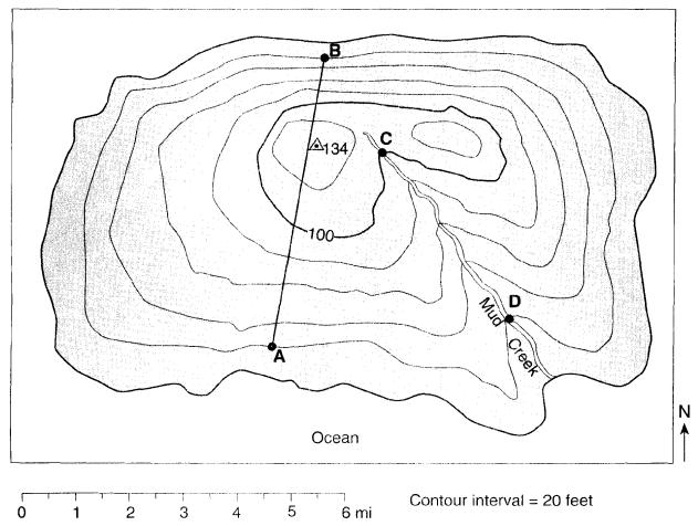
On the grid below, construct a profile along line AB by plotting an X for the elevation of each contour line that crosses line AB. Connect the Xs with a smooth, curved line to complete the profile.
